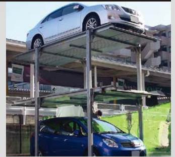
Mechanical parking lots
